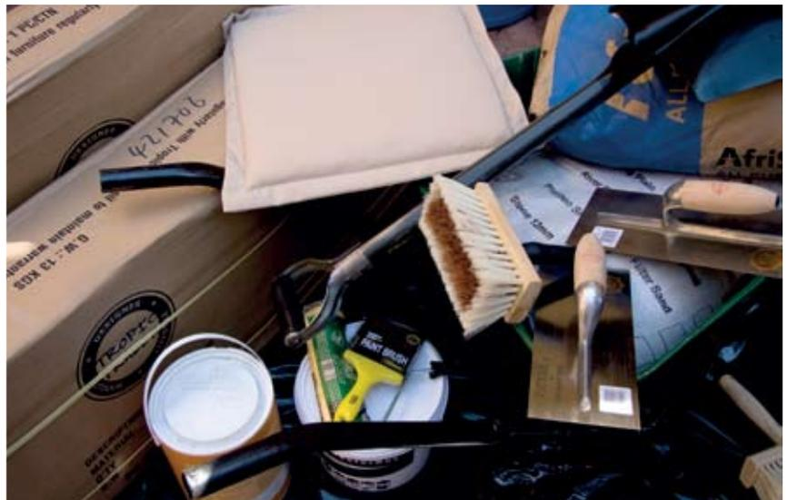
**'b**agging' cement is so named because of the traditional method of using a hessian cloth (or bag) to 'paint' a thin layer of cement over a facebrick wall or surface, while keeping the form of the bricks visible for visual impact and texture.
