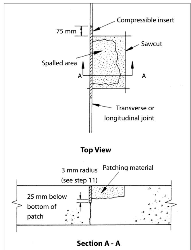
**Figure 1: Saw cutting at spalled joint**
