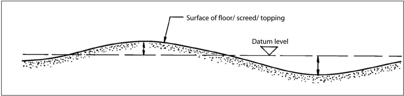
**Figure 1: Deviation from datum level (Exaggerated vertical scale)**
