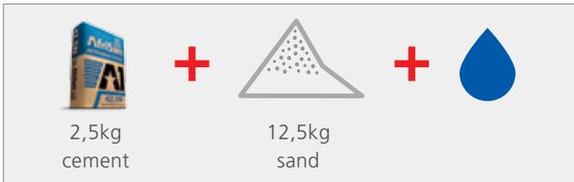
If more than three litres of water is required to make a workable mix, then the sand is unlikely to be suitable for plaster work.
